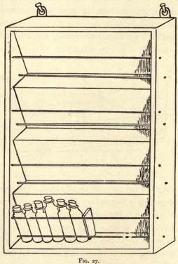
This form may stand on the laboratory table or can hang against the wall as desired. They can also be hinged together in pairs, labelled and placed on shelves.
