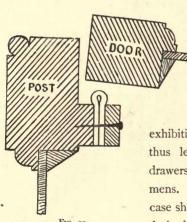
the joint all but airtight. The construction is readily seen from figure 23. The floor of a vertical case should be some few inches above the floor of the
