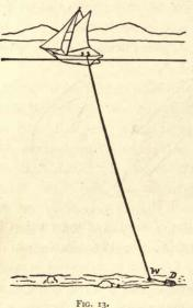
rope a short distance (six to twelve feet) in front of the dredge, so that its mouth may be kept on the bottom. The length of rope paid out should be about twice the depth of the water in which the dredging is conducted. In dredging from a sail-boat it is best, if possible, to take advantage of the currents. Put the dredge over the bows, taking care that it does not turn inside out
