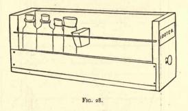
vials (one and two oz. can be admitted. The drawers may advantageously be four and one-half inches in depth and twelve inches in length. The bottles are fastened in position with a wedge as shown in fig. 28. These drawers may be placed together in a cabinet (fig. 29) and are interchangeable. By this means any desired arrangement of the collections can be effected, new specimens can be interpolated at any time and by having the drawers labelled any desired specimen can be at once found.
